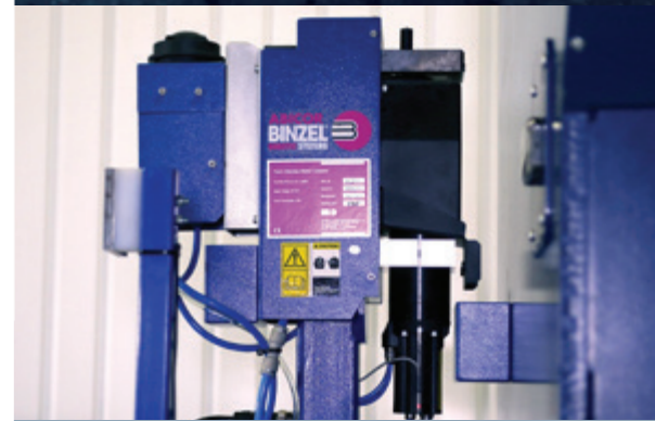
■ TORCH CLEANING STATION
