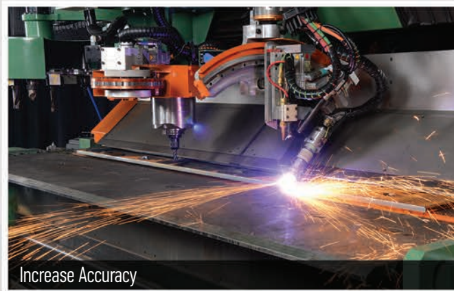
Bevel Cut 4" Thick Plate
