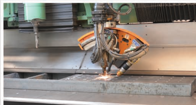
Bevel Cut 4" Thick Plate
